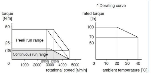
Dotted line represents the torque at 10 % less supply voltage.
