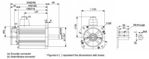
\* The external dimension is common between With or Without the brake.
