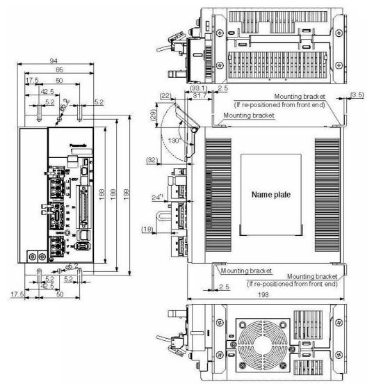
\*The external demension shown is for A5II and A5 series, but the demension is common between A5II, A5 series and A5IIE, and A5E series. Please refer to the catalogue for detail demension.
