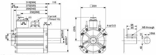
(a) Encoder connector (b) Motor/ connector (c) Brake connector (only with brake)
